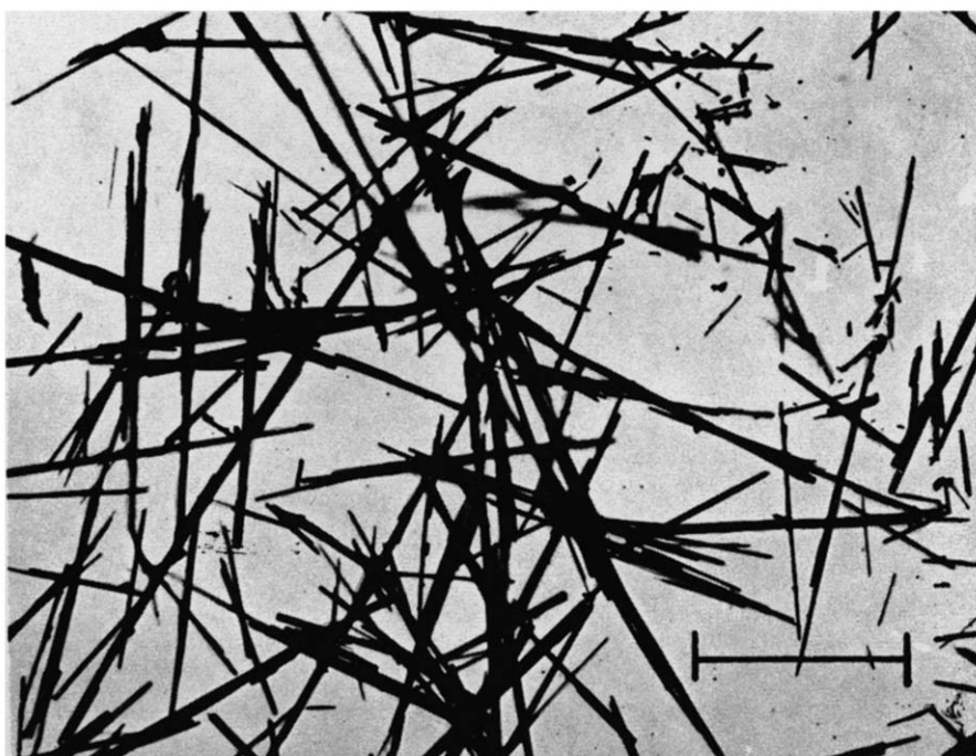
FIG. 2.—Nickel dimethylglyoximate precipitated from acetone-water solution.
