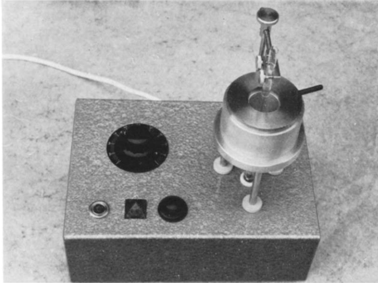
FIG. 1.—Ring oven plus variable transformer as a single unit (ROFA, Vienna, Austria).
