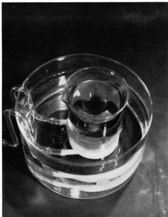
FIG. 3.—Stirrer operating whilst submerged in water bath.
